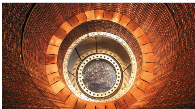
The ATLAS Hadronic Endcap Calorimeter (HEC). The HEC was constructed in Canada and assembled at TRIUMF. (Courtesy Roy Langstaff, University of Victoria/TRIUMF.)
