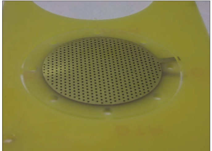
Fig. 1. A photo of a thick GEM showing the array of drilled holes.
